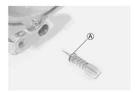
• Apply grease to the O-ring and install the accelerating plunger.
